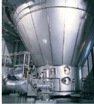
Conical part of CDP Dryer with powder outlet duct from the integrated fluid bed
