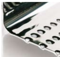
Sanitary T-profiles in the VIBRO-FLUIDIZER™
