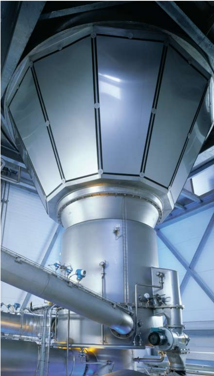
Integrated Filter Dryer - IFD™. Stationary fluid bed with back mix and plug flow section.
