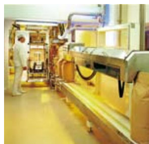
Bag heat sealing and belt transport
