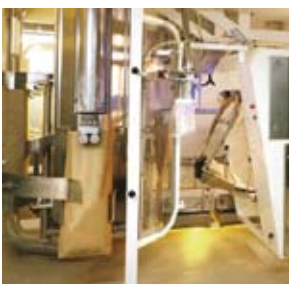
Automatic GEA Avapac carousel bagging-off equipment
