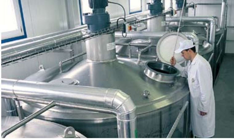
Whey crystallization tanks
