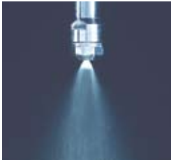
Pressure nozzle. Nozzle atomization results in good powder flowability
