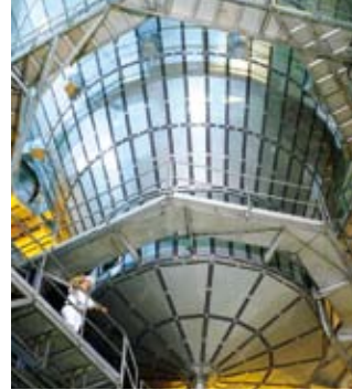
MSD™ Dryer with removable insulating panels
