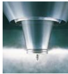
Rotating atomizer wheel in operation
